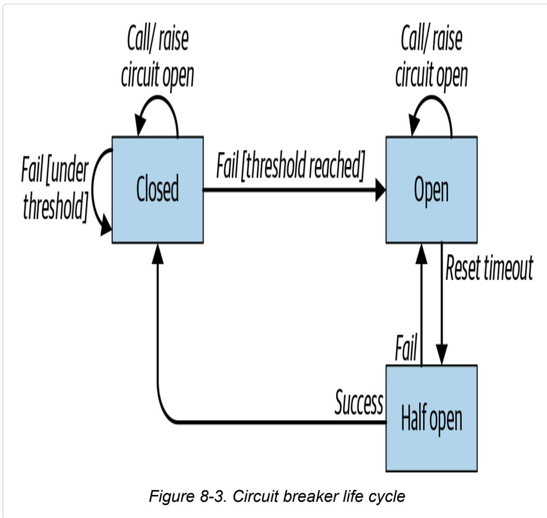
Figure 8-3. Circuit breaker life cycle
