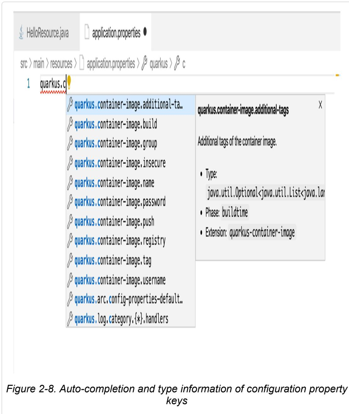
Figure 2-8. Auto-completion and type information of configuration property keys
