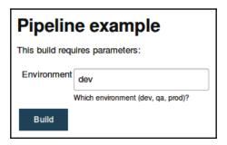
Parameterized build can help us reuse the pipeline code for scenarios which differ just a little bit. However, this feature should not be overused, because too many conditions can make the <code>Jenkinsfile</code> difficult to understand.
