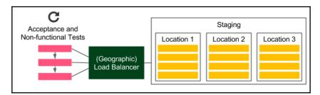
Note that the staging environment is an exact production clone. If the application is deployed in multiple locations, then the staging should also have multiple locations.
