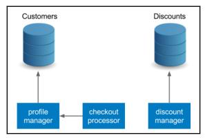
Such an approach is consistent with the principles of the microservice architecture and should always be applied. The communication over APIs is way more flexible than the direct database access.
