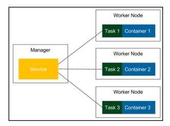
In Docker swarm mode, a running image is called a **Service**, as opposed to a **Container**, which is run on a single Docker host. One service runs a specified number of **Tasks**. A task is an atomic scheduling unit of the swarm that holds the information about the container and the command that should be run inside the container. A **replica** is each container that is run on the node. The number of replicas is the expected number of all containers for the given service.
