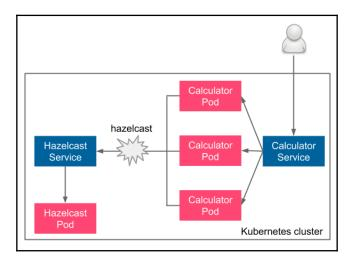
The user uses the Calculator Service, which load balances the traffic to a Calculator Pod. Then, the Calculator Pod connects to the Hazelcast Service (using its name, hazelcast). The Hazelcast Service redirects to the Hazelcast Pod.
