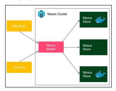
Apache Mesos, similar to other clustering systems, has the master-slave architecture. It uses node agents that have been installed on every node for communication, and it provides two types of schedulers:
