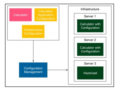
The configuration management tool reads the configuration file and prepares the environment, respectively (it installs dependent tools and libraries, and deploys the applications to multiple instances).
