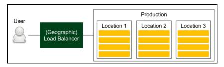
Users access the service through the load balancer, which chooses the exact machine. If the application is released in multiple physical locations, then the (first) device is usually a DNS-based geographic load balancer. In each location, we have a cluster of servers. If we use Docker and Kubernetes, it means that in each location we have at least one Kubernetes cluster.
